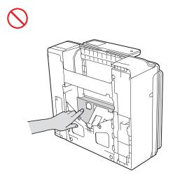
DO NOT carry the machine by holding the scanner cover, the Jam Clear Cover, or the control panel. Doing this may cause the machine to slip out of your hands and may result in injury. Carry the machine by sliding your hands into the handhold indentations located on each side of the machine.
